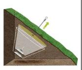
The second stage is where the anchor system is generating a frustum of soil immediately in front of the anchor. At this point load normally increases with minimum extension. The soil type will affect the overall extension.
