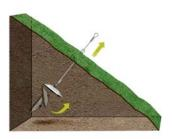
The first stage is where a load is applied to rotate the anchor into its loadlocked position. Elements of both load and extension are present.
