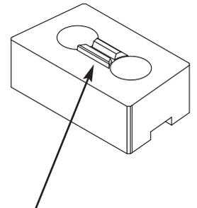
Easy-to-remove anchor bars let you cap walls quickly.
