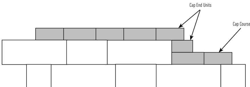
**NOTE:** To split a block, use a hydraulic splitter or split manually by using a hammer and chisel to score the block on all sides. Pound the chisel on the same line until the block splits. If partial unit sides are not exposed, use a saw with a diamond blade to achieve a tighter fit.
