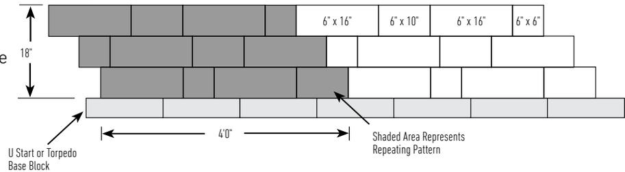
**NOTE:** These freestanding wall installation patterns show only one side of the freestanding wall. The same number of blocks are needed to build the other side of a freestanding wall when using Belair Wall 2.0 and Brisa freestanding wall systems. Freestanding wall installation patterns are measured in length by height of one side of the wall, and are expressed in square feet. Sets of blocks required include the number of blocks needed to build both sides of the wall.
