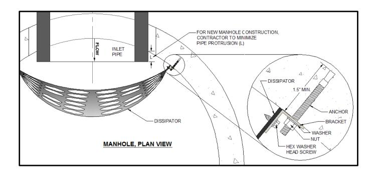
NOTE: Figure above illustrates an installed Preserver™ Dissipator.
