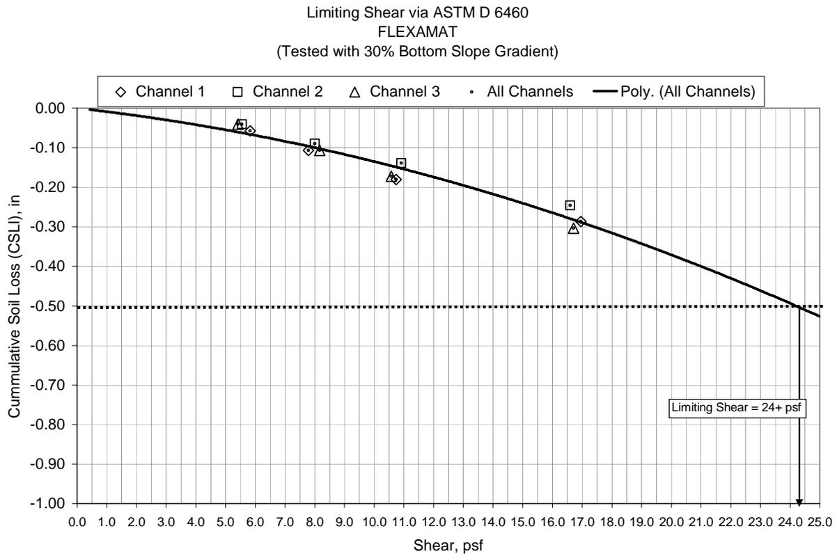
**Figure 11. Shear Stress vs. Soil Loss – Tested Product**
