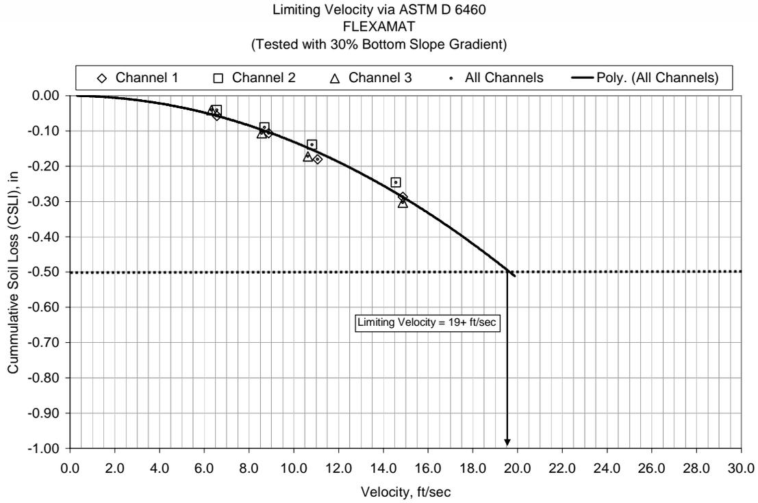
Figure 12. Velocity vs. Soil Loss – Tested Product
