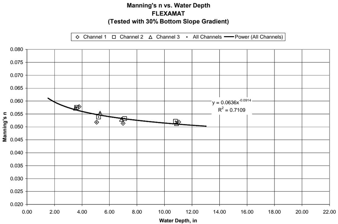
Figure 13. Roughness vs. Flow Depth – Tested Product
